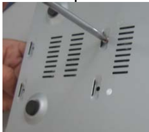
Fig 2.2 Screw HDD
