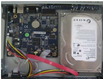
Fig 2.1 Connect HDD
